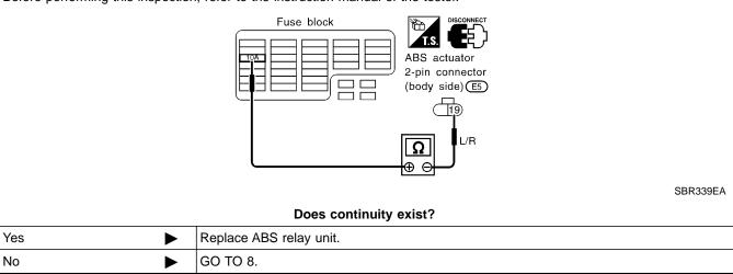
7. ABS Warning Lamp Stays On When Ignition Switch Is Turned On (Cont'd)
