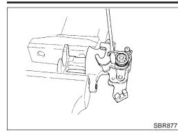
4. Remove return spring, toggle lever and cable guide.
