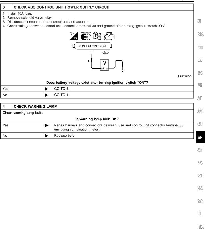
6. ABS Warning Lamp Does Not Come On When Ignition Switch Is Turned On (Cont'd)
